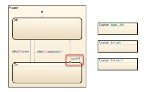
In the subchart, the transition path leading to the exit junction defines the logic for exiting the subchart. In this example, the function warm must evaluate to true on two consecutive time steps before the chart makes the transition out of the On state.
